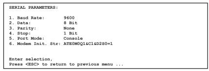
Figure 5.6: Serial Parameters Menu - Text Interface
